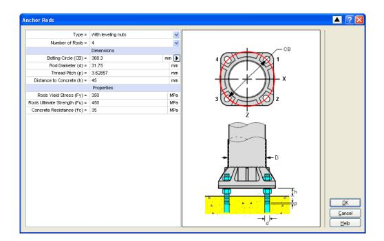
The arrow at the right of the **Bolting Circle (CB)** field allows to quickly select usual anchor rods parameter according to the diameter of the vertical support legs.:
