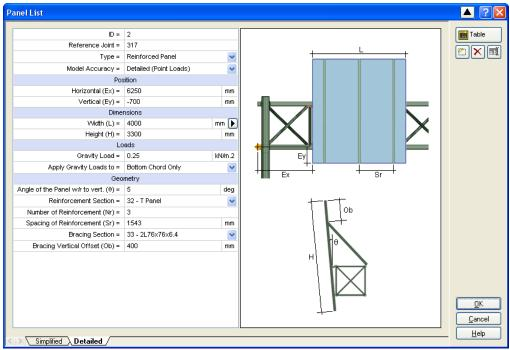
Note that the self weight and ice loads of the additional members generated in a detailed model add to the specified weight of the panel.
