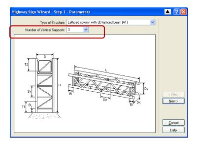
The additional support at axis 2 is located with respect to the first support by specifying its relative position from the center of axis 1
